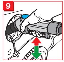
9. Once refuelling is complete, unlock the nozzle by pressing the trigger.
