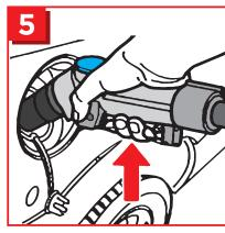
5. Insert the nozzle into the vehicle's filler neck and lock it into the refuelling position by pressing the trigger.
