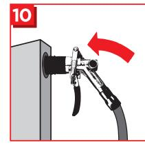
10. Remove the nozzle from the vehicle's filler neck and return it to the dispenser stand.
